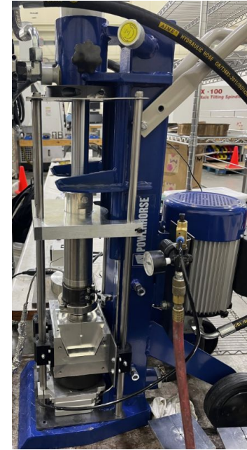
UMaine AMC custom built injection molder for test specimen manufacturing
